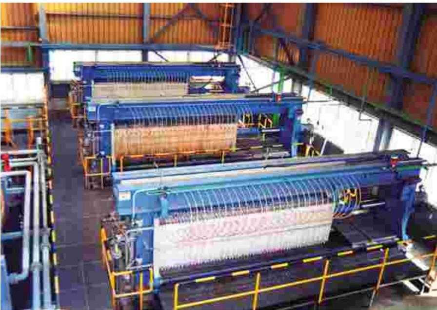
TEFSA has developed two systems in the range of the Overhead Filter Presses: the PEH and the PSEH.
