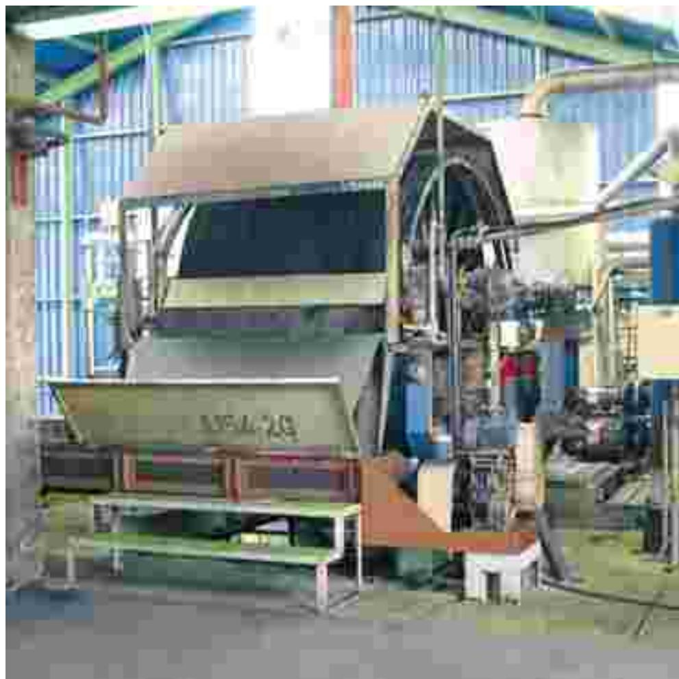
The TEFSA Vacuum Drum Filters are continuous filtration units, based on a drum partially submerged in a trough equipped with an agitator. The vacuum is given from the inner side of the drum. The continuous rotation of the drum allows the unit to filter the product, wash the cake, dry the cake and discharge the cake without interruption necessities, only adjusting the rotation speed to the characteristics of the product.
