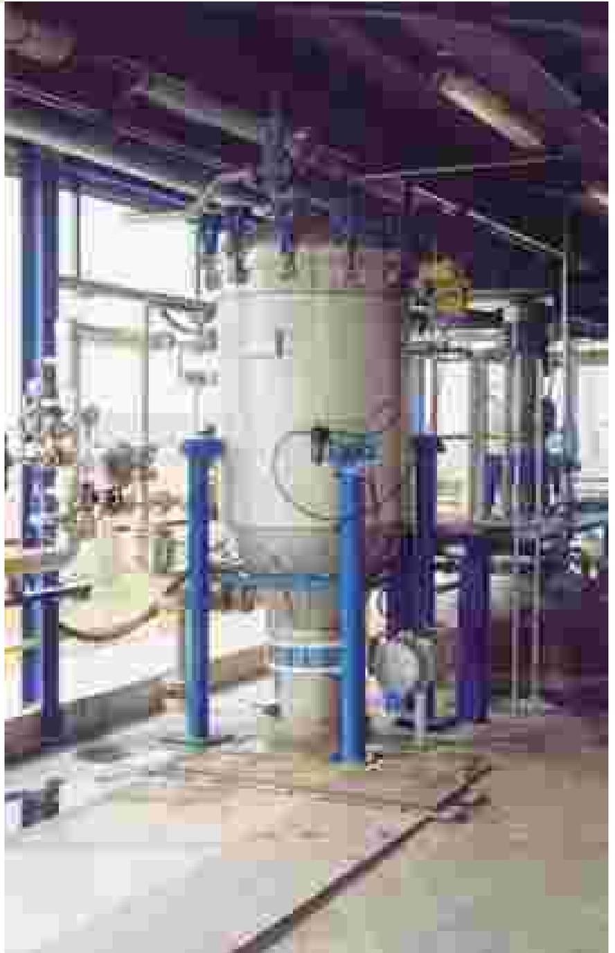
Being the filter of closed and watertight execution, it is commonly used for the treatment and filtration of dangerous liquids and/or of high value, achieving a complete liquid squeezing and operating by batches with absolute nonexistent product loss.
